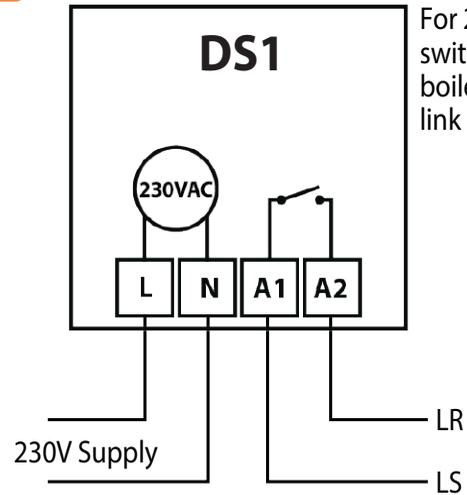
LS & LR ARE NORMALLY THE ROOM THERMOSTAT CONNECTIONS
