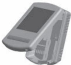
Carefully separate the front half of the thermostat from the back plate by placing a small flat head terminal driver in to the slots on the bottom face of the thermostat.
