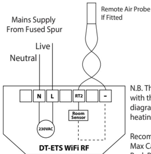
N.B. The DT-ETS WiFi RF is designed to work with the RC2-W. Please refer to the appropriate diagram for connections to your heating system.
